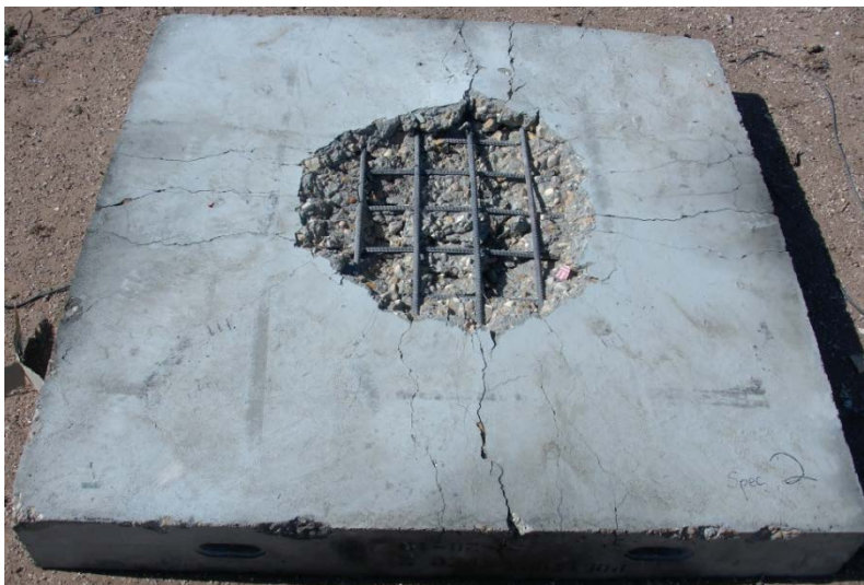
Figure 5 Panel 2 (Control) - 7lb of C4
