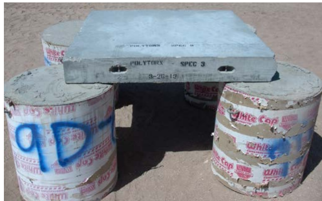
Figure 2 Breach testing panel support
