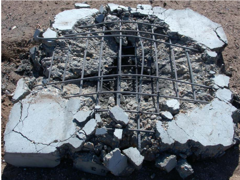
Figure 4 Panel 3 (Control) - 10lb of C4
