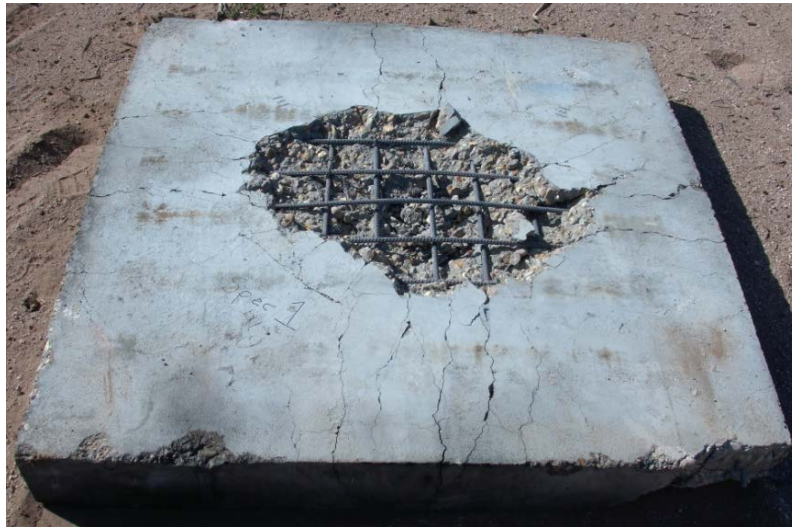
Figure 6 Panel 1 (Control) - 8lb of C4
